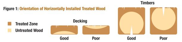
**Material size** – for decking surfaces in non-residential applications such as docks, boardwalks, and commercial decks, full 2" or even 3" thick decking material should be used for extra durability.
